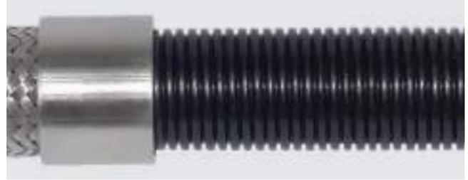
When electrically resistive fluids like solvents and fuels, or multiphase mixtures are passed through natural PTFE hose at high flow rates, a static charge build up occurs on the inner wall of the PTFE liner. This can discharge to the nearest conductor (e.g. SS braid) that creates a pin-hole in the PTFE liner resulting in a leak-path.
