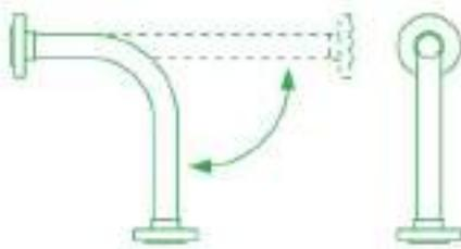
**CORRECT** - Flexing movement takes place in 2 dimensions
