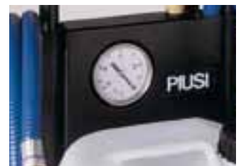
Suction pressure and operation check.
