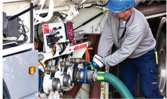
The self sealing design of the Dry disconnect couplings guarantees both the highest level of safety and also the quickest way of connecting and disconnecting.
