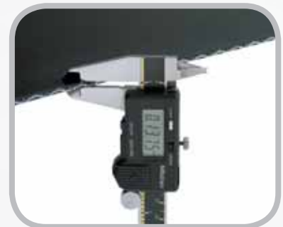
Measure belt thickness.
